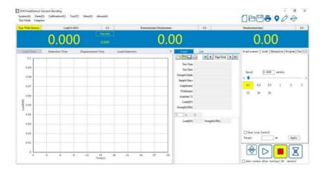
• Curve drawing: The software system provides abundant test curve display. Such as forcedisplacement curve, force-deformation curve, stress-displacement curve, stress-deformation curve, force-time curve, deformation-time curve.
