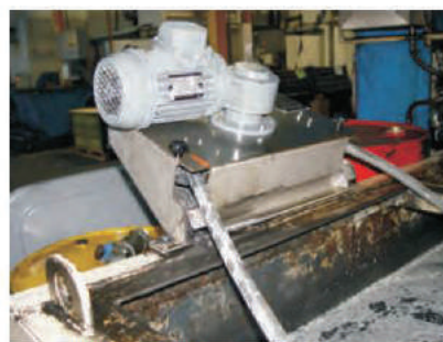
Oil skimmer model W40 at coolant tank
