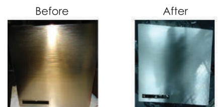
Hair Line Mold Ultrasonic + Electrolysis 12 minutes
