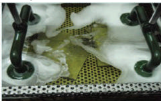
Cleaning Process with Ultrasonic + Electrolysis Only
