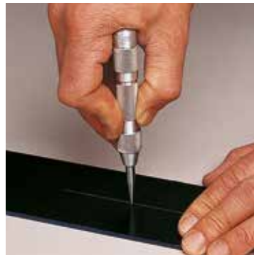
Easy one-hand precision centre punching
