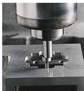
Above left: Locating the centre with 827MB Left: Locating the edge of a part with 827MA
