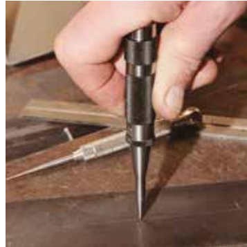
Rugged automatic centre punch with adjustable stroke
