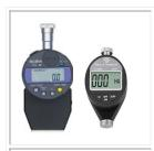
Digital Durometers (Rubber Hardness Testers) 0-100 degree (up to 45000mN / 4533gf)
