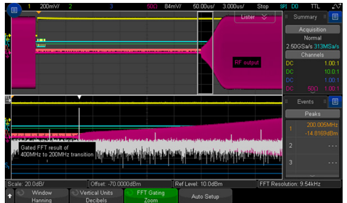
Figure 21c. Start observing the RF signal at 200 MHz. You can validate this from the RF analog waveform as well.
