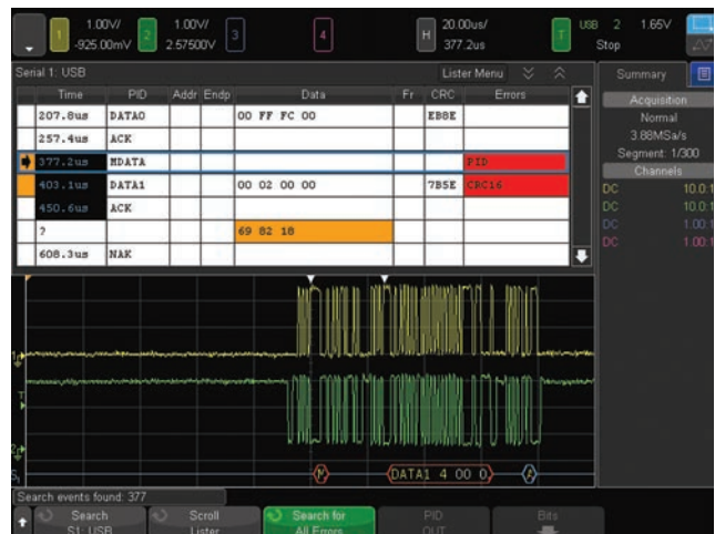
Figure 21. USB 2.0 trigger, decode and "lister" display.
