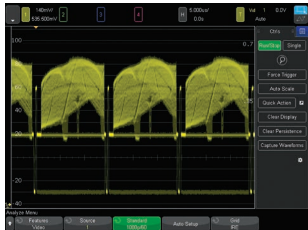
Figure 27. Triggering on 1080p HDTV signal analysis.
