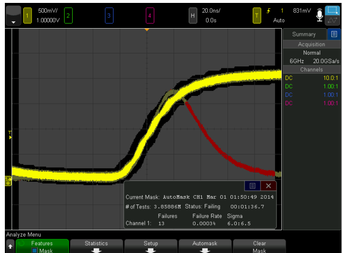
Figure 40. Limit testing of infrequent glitch.
