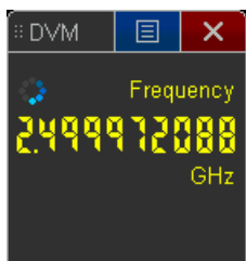
Figure 32. 10-digit counter making precise frequency measurement on a 2.5-GHz signal.
