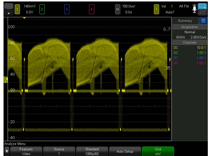
Figure 45. Triggering on a 1080p/60 signal.
