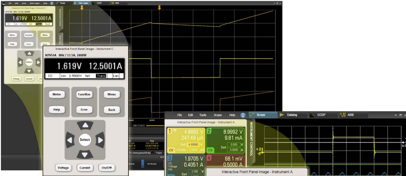
14585A connected to an N7954A
