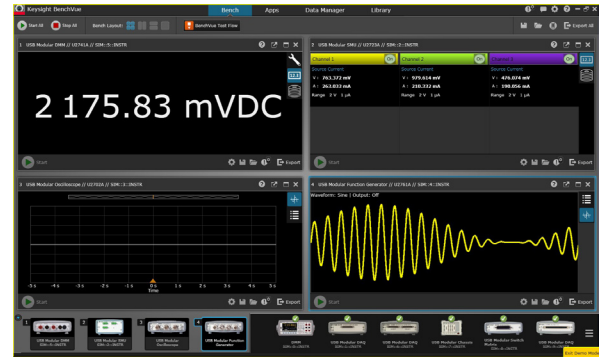
View measurements across USB DAQ, modular and bench instruments all on one BenchVue interface.
