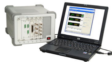
U2722/3A used as a modular instrument
