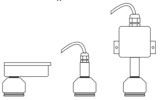
**WARNING:** Do not flip over calibration vessel with applied humidity standard – the only allowed position is with lid downwards (see figures)!
