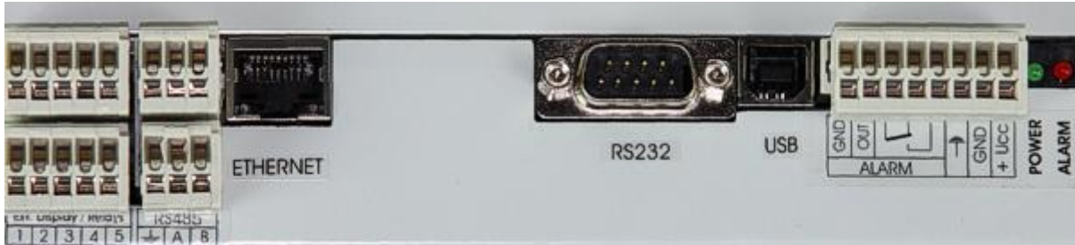
Figure: communication interface, alarm outputs, connection of power. Ethernet interface is optional.
