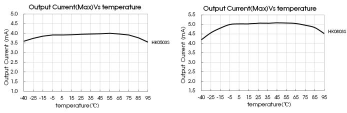
Note: In the curves, the maximum output current is typical value in different temperature.
