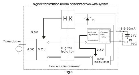
Due to the potential risks based on the different ground, you can isolate the MCU and the current loop DAC and HART modulator by digital isolation. Current loop DAC and HART modulator is floating form. They make the high impedance formed to two ground potential between two-wire instrument and PLC system, and reduce the loop current between the ground wire, So that two systems are isolated and the hidden trouble of common mode interference is eliminated.
