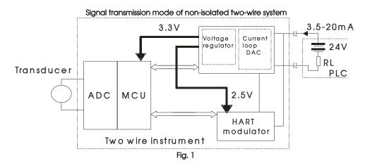
In the circuit of fig. 1, Sensor signal is converted into digital signals through the ADC, then sent to the current loop DAC and HART modulator through MCU, and form 3.5~20 mA signal output. Current loop DAC get power supply from the PLC bus of output 3.5~20 mA, and output 3.3 V and 2.5 V through the built-in voltage regulator, supply a small amount of power for MCU and HART modulator.
