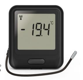
During configuration, the sensor will search for an existing wireless network whilst physically connected to the PC. It can then be placed anywhere within range of the network. If the sensor temporarily loses connectivity with the network, it will log readings until it is able to communicate again with the PC application or FilesThruTheAir™ Cloud (max 30 days at 10 second sample interval).
