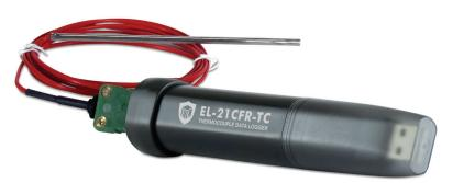
This standalone data logger measures and stores more than 32,000 temperature readings from a J, K or T-type thermocouple at a resolution of  $0.5^{\circ}$ C (1°F). It comes supplied with a K-type thermocouple capable of measuring from 0 to +200°C (32 to +392°F).
