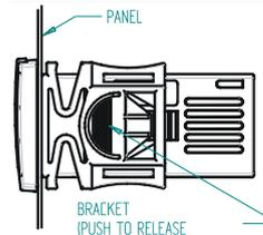
Instrument XR03CX and XR04CX shall be mounted on vertical panel, in a 29x71 mm hole, and fixed using the special bracket supplied.
