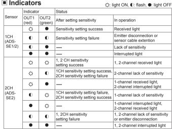
$\frak{K}$  For ADS-SE2, OUT1 indicator(red) is for Receiver status set sensitivity by Emitter of 1-channel and OUT2 indicator(green) is for Receiver status set sensitivity by Emitter of
