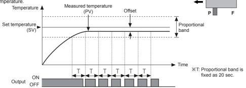
It is available to control without overshoot or hunting comparing ON/OFF control but it may cause offset. Correct the offset with the RESET volume switch.
