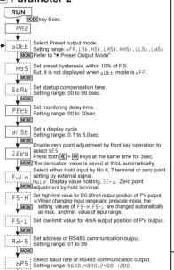
Advance to the parameter to be changed when pressing MODE key continuously in RUN mode and releasing MODE key at the parameter. (Refer to "a Parameter Setting") When pressing MODE key in each parameter, the initial mode of the parameter is displayed. (Refer to the description of each parameter.)
