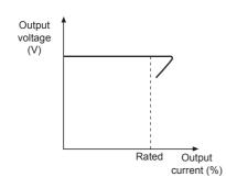
• It is able to protect over current by load with built in over current protection circuit. When the over rated current is flowed, the circuit is operated (output voltage is fallen) and it is released when the load current is under the rated current (it is returned to the rated output voltage).
