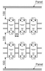
%For mounting multiple SSR, please keep certain installation intervals for heat prevention. For horizontal installation (when the heights of input part and output part are equal), it is recommended to apply 50% of rated load current.
