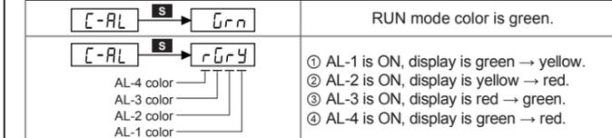
• When alarm is cleared, or two alarms operate at the same time, the latest alarm's color is applied.
