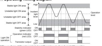
\*The waveforms of "Operation indicator" and "Transistor output" are for Light ON operation They are reversed for for Dark ON operation.
