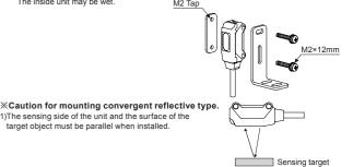
2)Make sure to install the sensor after carefully considering the moving direction of the sensing objects
