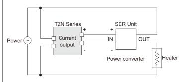
•It is important to select SCR unit after checking the capacity of the load. •If the capacity is exceeded, it may cause a fire.
