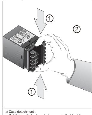
Pull the handle backward after press both side of it on terminal block
