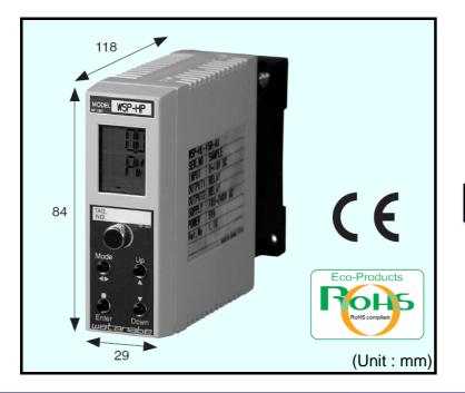
This compact plug-in converter receives DC signal input and outputs a relay contact signal or open-collector signal if the DC signal input value exceeds the preset value (one point).
