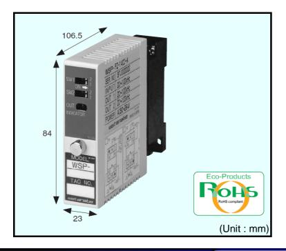
This compact plug-in converter (pulse isolator) receives a pulse train signal extracted from the sensor or control equipment, adds waveform shaping, insulation, and level conversion, and then outputs two pulse string signals.
