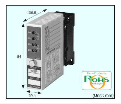
This compact plug-in converter accepts AC voltage or current input and provides optically isolated two DC voltage or current outputs. Since WSP-EFW type adopts the true root-mean-square value operation system, it ensures particularly high reliability against distorted waves.
