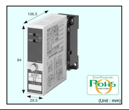
This compact plug-in converter accepts AC voltage or current input and provides optically isolated DC voltage or current output. Since WSP-EZ type adopts the true root-mean-square value operation system, it ensures particularly high reliability against distorted waves.
