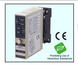
This compact plug-in, high-speed response type converter (isolator) provides 2 signal outputs which are mutually isolated between input, output and power-supply. It amplifies and converts various kinds of signal with isolation to use in the integrated instrumental control system. It is highly effective as noise countermeasures.
