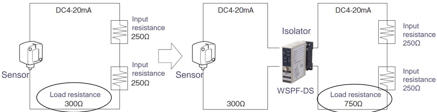
Correct current does not flow when load resistance of sensor output is not enough.
