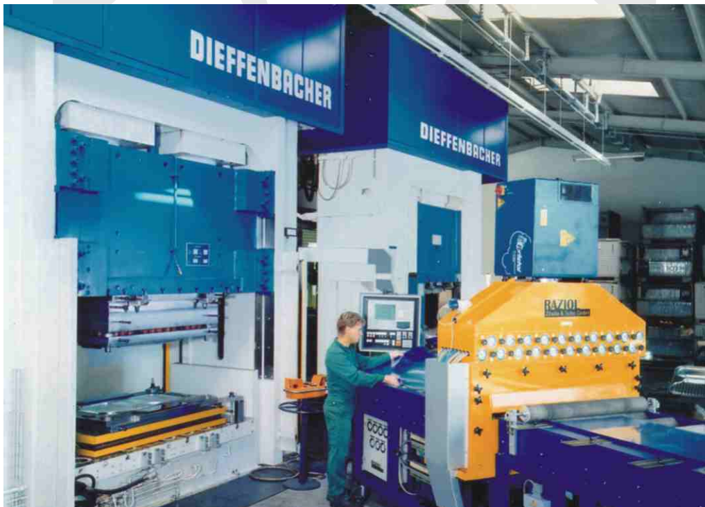
Converter Press with a laterally fitted greasing station (Maschinenfabrik J. Dieffenbacher GmbH & Co., D-Eppingen)
