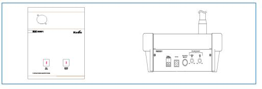
**RM5001** shall be used when a direct paging is required without having to select zone or when paging is to be made near rack which is installed with zone selector. It is also used as emergency paging console as a dry contact is available whenever the mic is active which is used to activate **ALL CALL** or overriding or as any other emergency contact.
