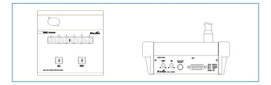
**RM5006** shall be used when paging to specific zone is required in which the main rack is located away from the paging station.
