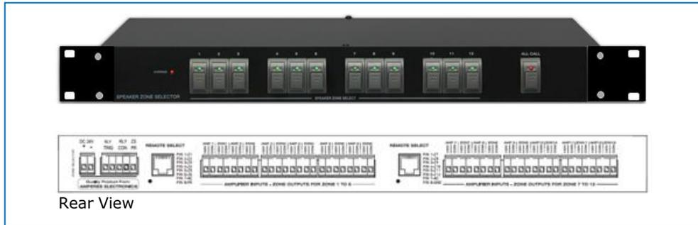
Available in 12 zone version, used for selecting speaker zone directly via the front panel or from remote paging console.
