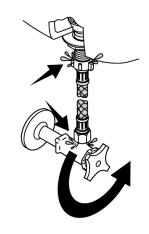
6. Fix the WDI Fitting according to Manufacturer installation manual. If needed, adjust the tank water level. Then Install the seat and tank lid.
