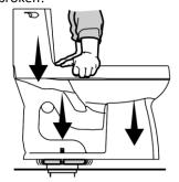
3. Install the washers and nuts as shown. **Do not over tighten!**
