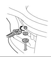
4. If needed, cut off the T-bolts before installing the bolt caps (not provided.
