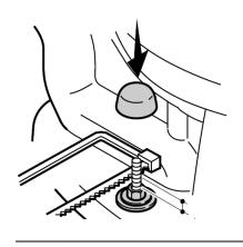
5. Connect the water supply and turn on the valve. Check for leaks. **Do not over tighten!**
