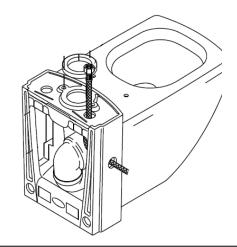
6. Install the dual-flush button into the lid. Carefully place the tank lid into the tank where the flush button is accurately on top of the WDI fitting. Finally install the seat cover provided.
