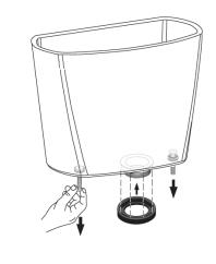
4. Carefully place the water tank on the seat and tighten the screw. Ensure the correct position of the sealing ring into the valve nut.
