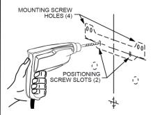
4. Fix hanger to wall (loose). Mount basin for positioning, level the deck, and mark bottom anchor screw holes (if applicable). Remove basin, tighten the hanger positioning screws and drill pilot holes for anchor screws and 4 mounting screws. Install and tighten the mounting screws.
