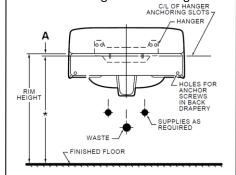
3. Drill pilot holes in positioning screw slots of hanger.
