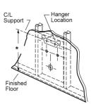
2. Determine the desired rim height Position hanger making sure its centre is aligned with the waste hole centreline. Mark the hanger screw locations through its mounting holes.
