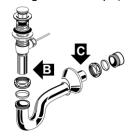
6. Connect hot and cold supply lines to the shut-off valves. Tighten trap joints for watertight assembly. Apply a bead of caulk around the edge which contacts the wall.
