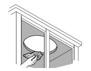
5. Place the basin under the opening. Hold the sink in place and rotate each clip over the ring and then even tighten the clip to secure.
