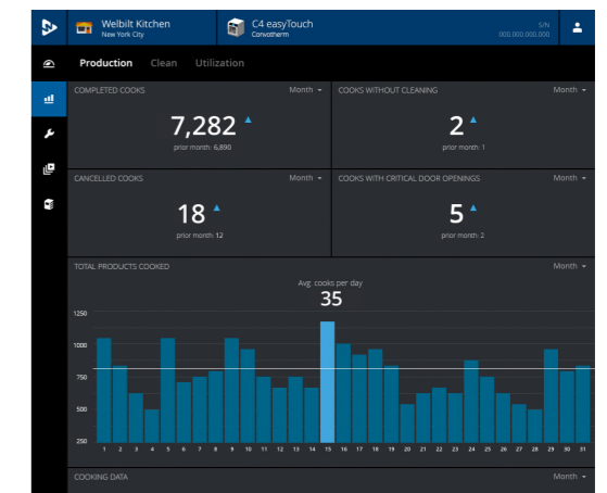
Display of events with relevance for quality, such as omitted cleaning cycles or canceled cooking processes.
