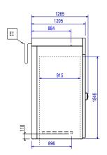
Drain ΕI Electrical inlet (power) Refrigerant Outlet
