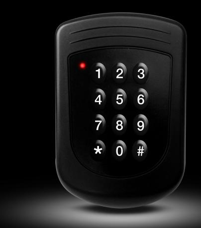
RD.BA3028 Proximity Reader is a fully self contained proximity access controller, used as standalone device without personal computer connected
