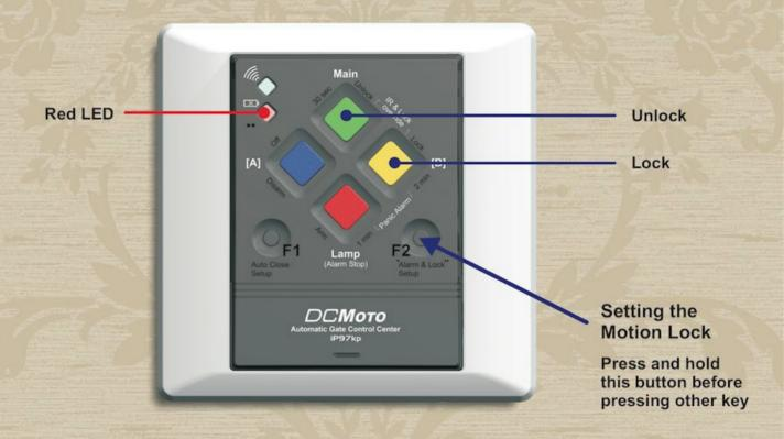
If you press the setup button F1 + F2 together and the red LED lights up, it means the MOTION LOCK is active. The light is off if it is unlocked
