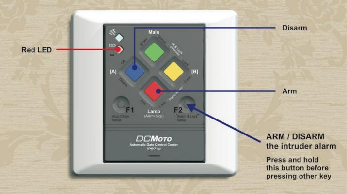
If you press the setup button F2 and the red LED lights up, it means the alarm is ARMED. The light is off if the alarm is DISARMED
