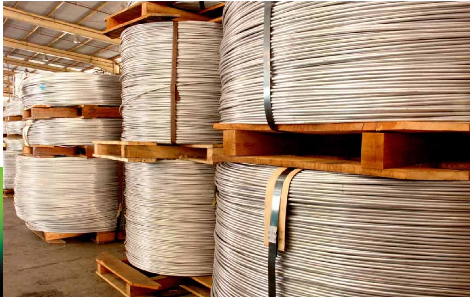
Aluminium and aluminium alloy electrical conductors are made by various processes from wire-drawing (i.e. rod breakdown to fine wire) to wire stranding from a large diameter of redraw aluminium and aluminium alloy rods.
