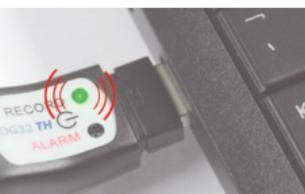
Connect logger to USB port. Beeper sounds for 1 second. The recording stops. LED blinks green until result PDF is created (can take up to 40 seconds).
