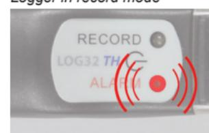
Beeper sounds once each 30 seconds for 1 second, red LED blinks each 3 seconds - measured values exceeds selected measurement range (not with standard settings). Alarm limits can be changed using LogConnect\* software.
