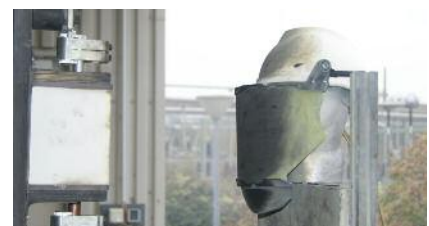
GS-ET-29 class 2-7 kA certification passed. Head and face combination protects the wearer
