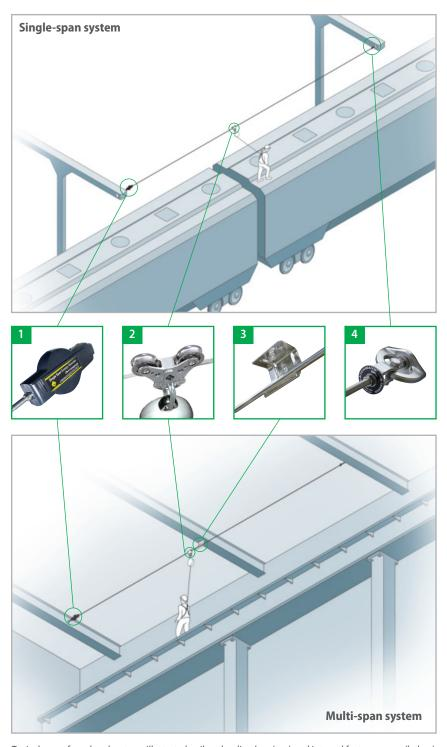
$\label{thm:continuous} \textit{Typical uses of overhead systems illustrated: } \textit{rail car loading bay (top) and internal factory access (below).}$
