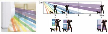
FMX has 78 dense zones to cover the whole detection area. At any spot within the detection area more than 4 (quad) zones are utilized to verify if it should generate alarm or not. Also The CORE platform enables the QUAD ZONE LOGIC to evolve to the next step. providing digital quantification of infrared energy, FMX enhances accuracy in both human detectability and pet immunity.
