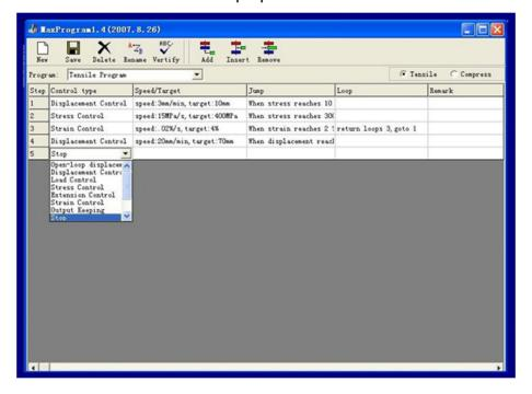
Through the Tensile Program Editor, user can setup test steps according to the requirements of standards.
