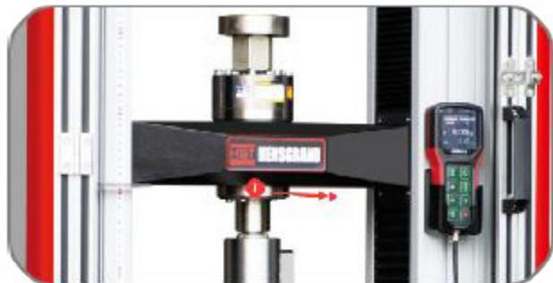
**Installation of indicator ruler :** for real-time observation of the position of moving beam The limit switch adopts the built-in installation mode, the outside adopts the limit adjusting rod and the position locking knob, has the strong sensitivity. Safe and reliable.
