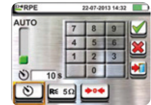
Selection of AUTO or TIMER measuring mode
