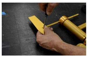
The wind speed and direction sensor is shipped with tail removed, replace and tighten screw.
