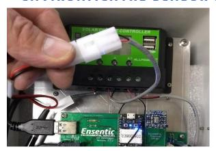
Only after all sensors are attached you can connect the battery
