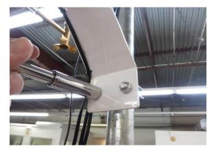
Attach Temperature/Humidity sensor with saddle bracket and tighten with ½ socket wrench
