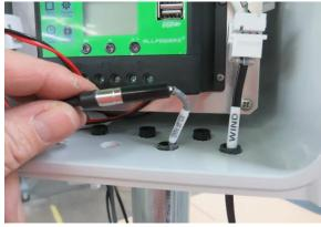
If equipped connect the solar panel connector.
