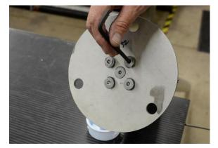
Screw in partially the center screw, the remaining screws, then tighten
