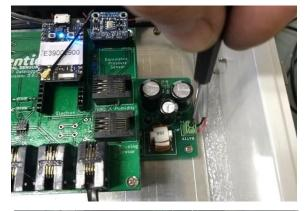
If powering with 12VDC. Make the power connection to the PCB at this terminal. + positive is marked BATTP and the – is marked BATTN.
