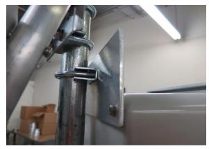
Attach the control box to lowest part of upper mast section and attach with saddle brackets
