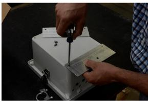
Unbox you're the controller. Remove the brackets from back side and rotate and reattach
