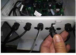
tighten with O-rings, sealing for water tight connection
