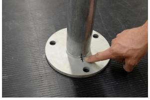
Align mark to ensure bolt hole pattern matches
