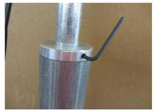
Assemble the wind sensor
