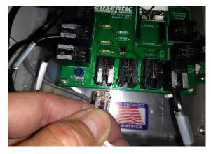
Connect each sensor to appropriate socket, all should be marked
