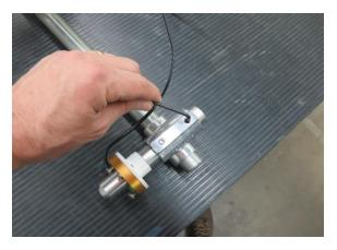
Assemble the solar sensor if equipped
